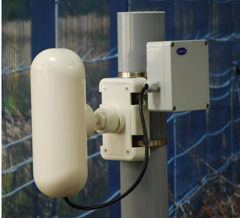
Drawing 1.2 – Setting up the RU (TU) and the optional DB on the stand
